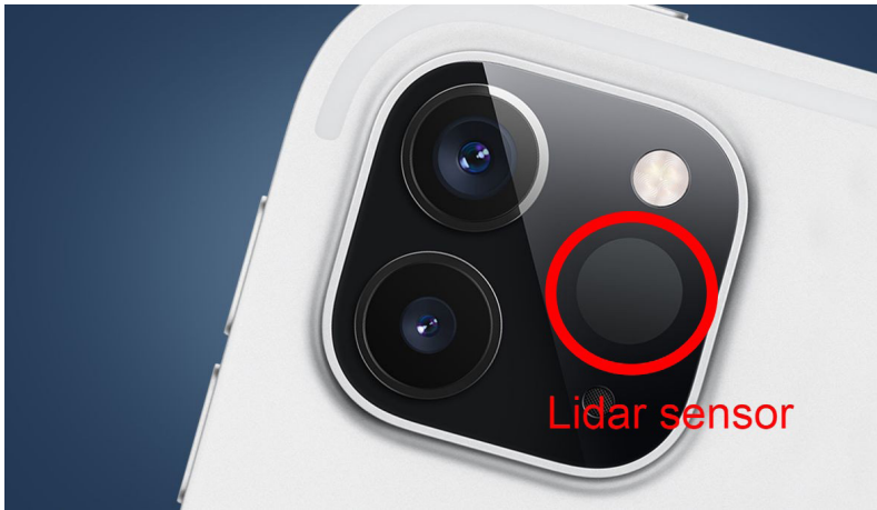
Figure 1: Position of the lidar sensor in the Apple iPad Pro 2020 (source: own photography)
