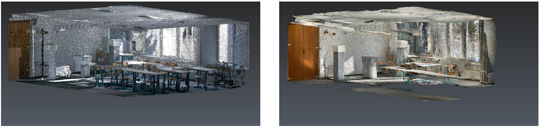
Figure 7: The point cloud of the larger test field captured with the BLK360 scanner (left) and the Apple device (right).
