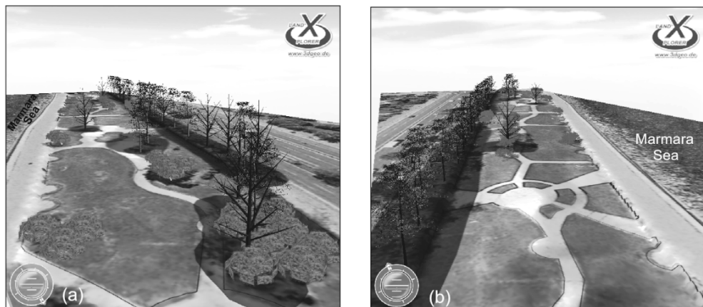
Figure 6: The combination of the aerial photo and RTK GPS/GLONASS measurements in the project area (3D digital terrain model of the project area), (a) is north-south direction, (b) is south-north direction
