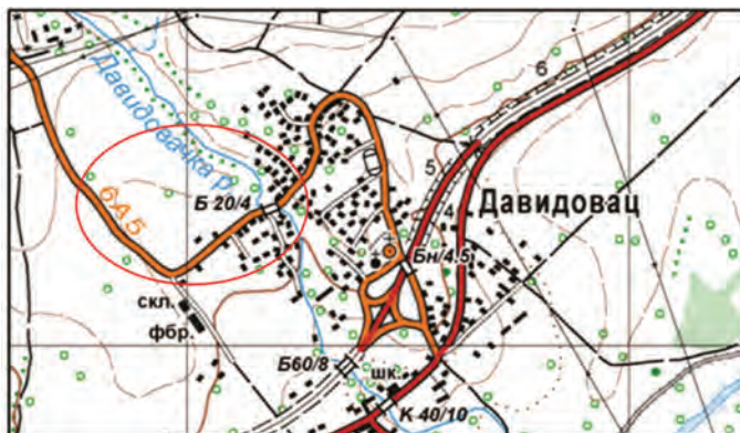
Figure 4: Defined annotations on the road infrastructure.
